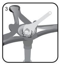
Tighten the bolt with a spanner.
