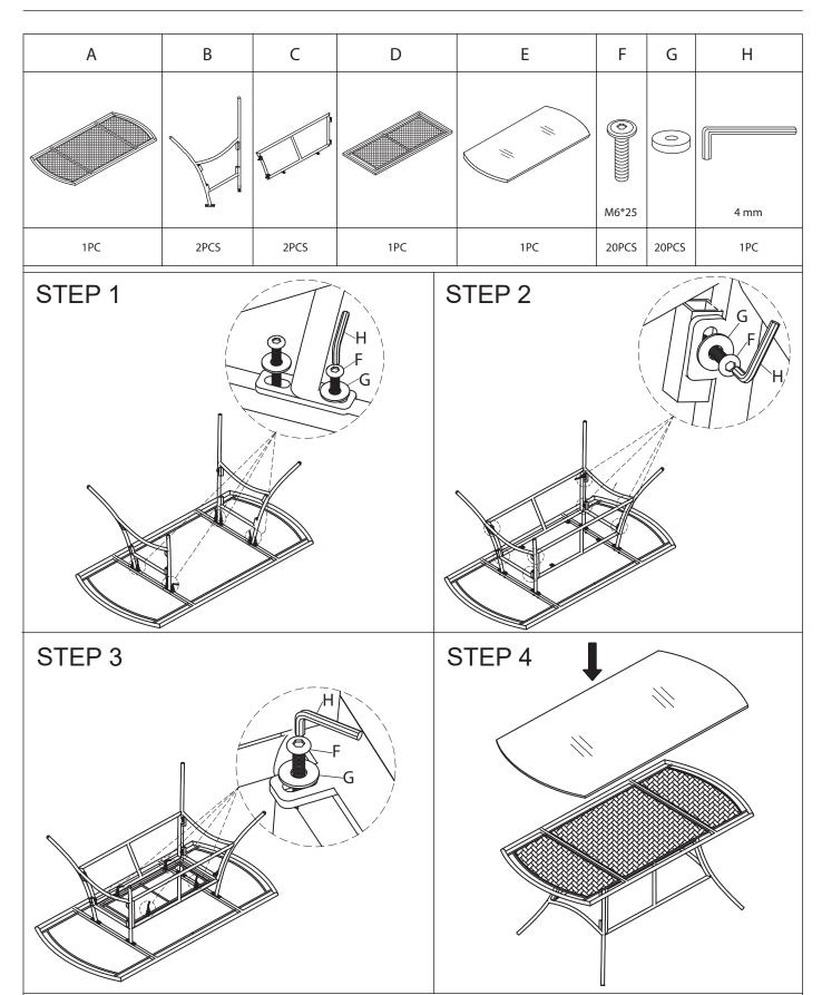
Remark: Be noted, during assembly, we recommend only to tighten all screws with 80% fastening, when having all screws in correct position, and tightened to 80% - then OK to tighten to 100%, to avoid any distortion, bendings.
